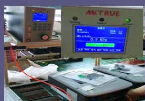
Air tightness test
